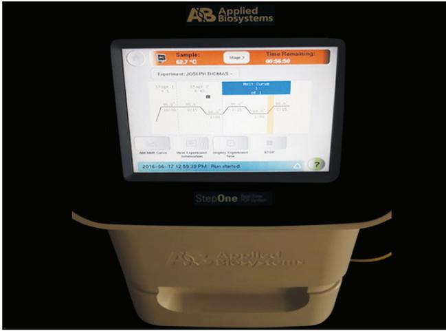
Fig. 3: Real-time PCR machine running the protocol for species evaluation
