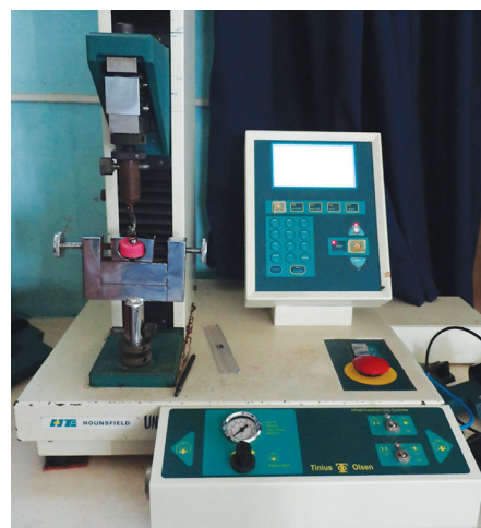
Fig. 1: Specimen undergoing retentive strength testing in Instron universal testing machine
