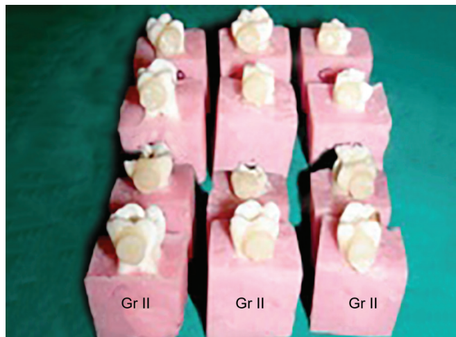
Fig. 2: Composite cylinders built-on prepared specimens in samples of group A2
