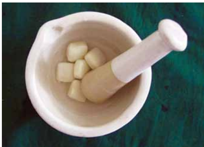
Fig. 1: Five chewing gums with 25 ml of artificial saliva (5 ml of artificial saliva/chewing gum)
