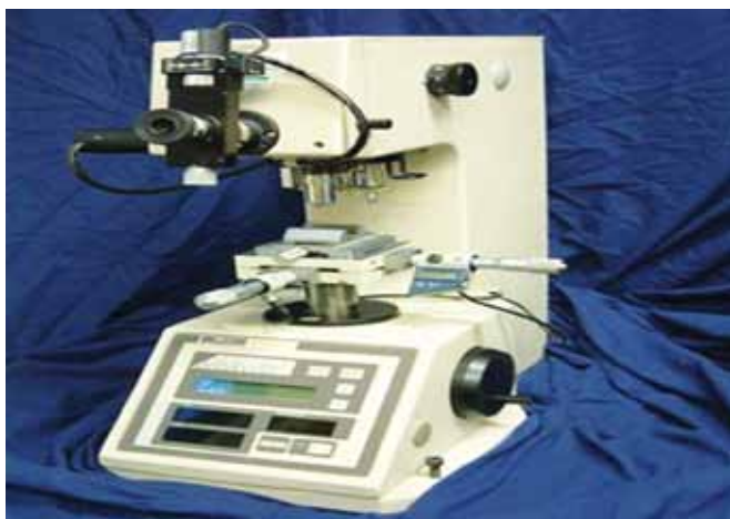
Fig. 5: Knoop microhardness indenter
