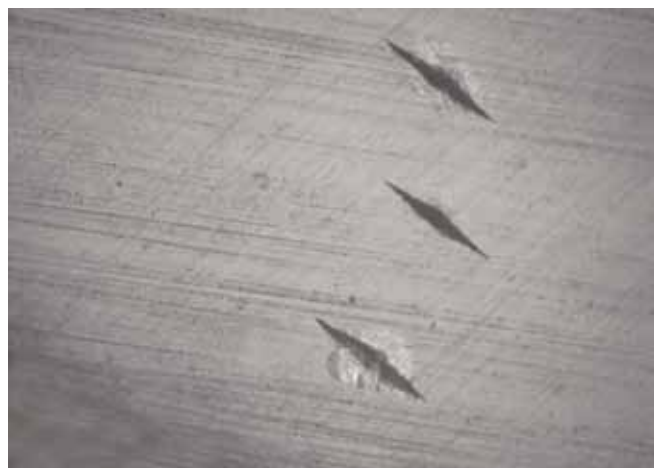
Fig. 6: Three knoop microhardness indentations
