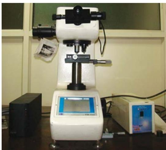
Fig. 4: Vickers hardness tester (Future-Tech Corp FM-700, Tokyo, Japan)
