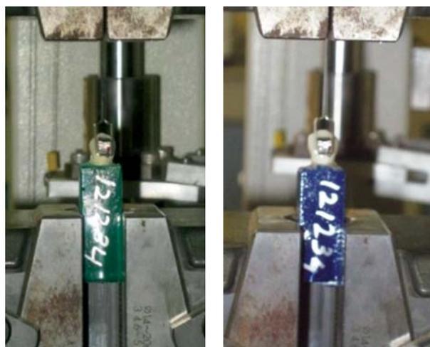
Fig. 2: Aluminum cubes placed in lower clamp (Fixed Head) of the universal testing machine
