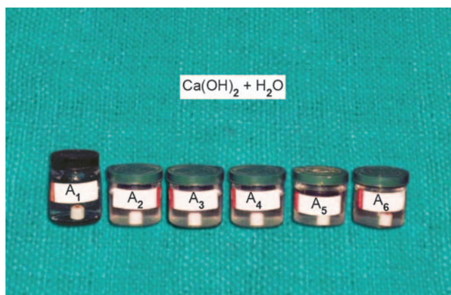
Fig. 4: Six bottles containing 40 ml of distilled water with porcelain caps immersed into it having a paste of a \text{Ca}(\text{OH})_2 + \text{H}_2\text{O}
